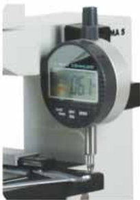
pic. 23: indicator gauge for depth measurement
